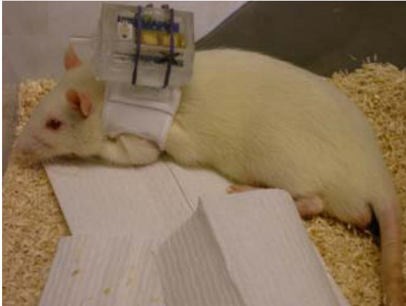
Fig. 6 The pumping system were connected to the rat through a backpack [17]
