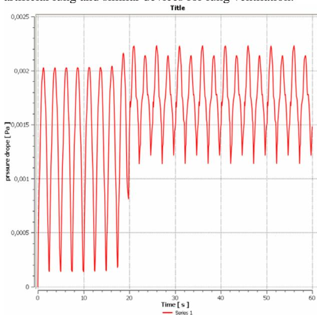
**Fig. 9 Pressure drop in the domain**
