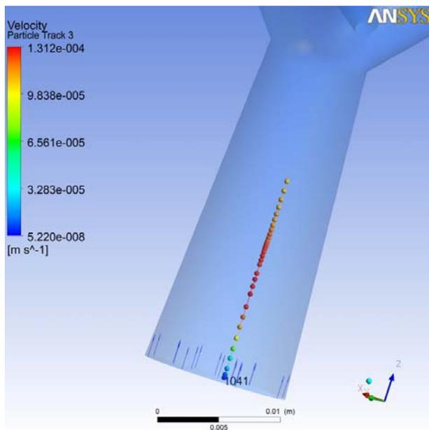
**Fig. 11 Positions of the particle along its tracking line colored by velocity magnitude**
