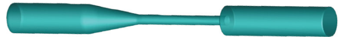
Figure 2 Tube with sudden expansion used for the FDA Critical Path project [6], with blood flow from left to right.
