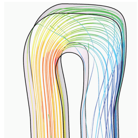
U-bend optimized for minimal pressure losses
