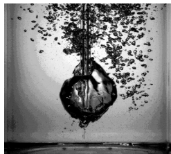
Experimental simulation of lance bubbling
