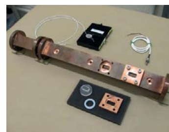
CHIEF Facility test section representative of a real rocket engine cooling channel
