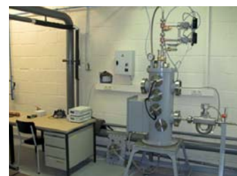
CHIEF Facility configured for cryogenic two phase flow characterization testing
