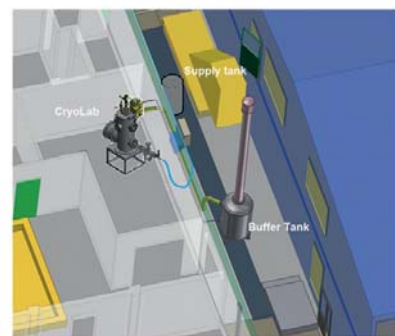
Representative view of the CHIEF location inside the Cryogenic Laboratory at VKI with the related LN2 supply and LN2 evacuation installations
