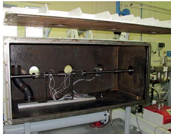
CryoLine Facility configured for valve characterization testing
