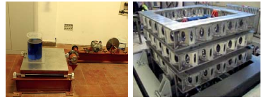
(a) Small sloshing table (b) Shakespeare table Figure 1 - Sloshing facilities at VKI
