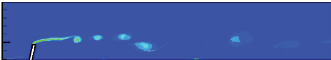
LES Simulation of vortex shedding behind the deformed PT
