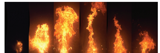
Flame enlargement during Boilover (Dt=0.2s)
