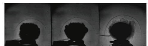
Shadowgraph of BLEVE rupture with 80mm weakness (left), 40mm (middle) and 10mm (right)
