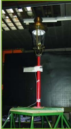
Wind resistance test on lantern
