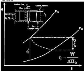
Figure 1: Enthalpy-entropy diagram of a gas expansion in a turbine; Definition of the control volume and the flow quantities that influence the turbine efficiency; simple efficiency definition
