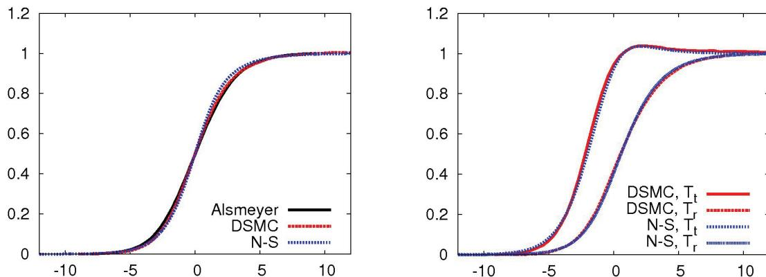
**Figure 1 : Mach 1.71 shock wave: comparison between CFD and DSMC solutions, normalized profiles of density (left) and temperature (right)**
