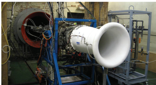
Figure 1: VKI Cooled Probe installed on RR Viper before and Engine, and the cooling system (right) installation (center)
