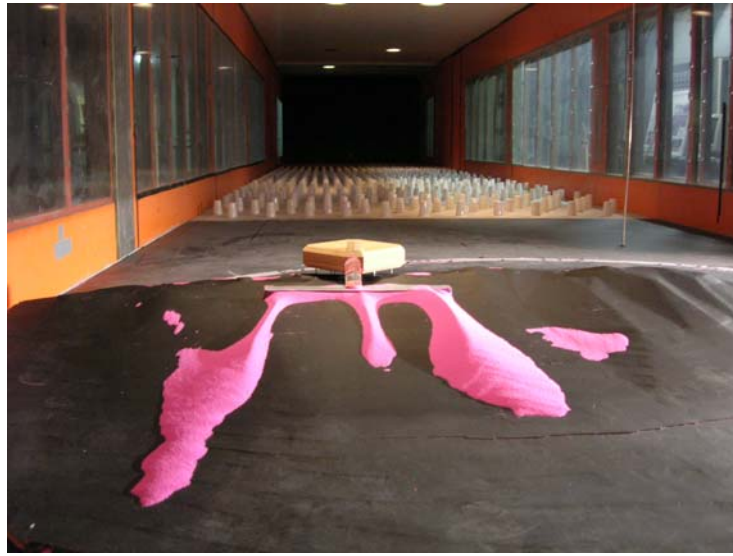
Figure 4: Wind tunnel testing of snowdrifts using sand (VKI L1-B wind tunnel: 2m high, 3m wide and 20 m long)
