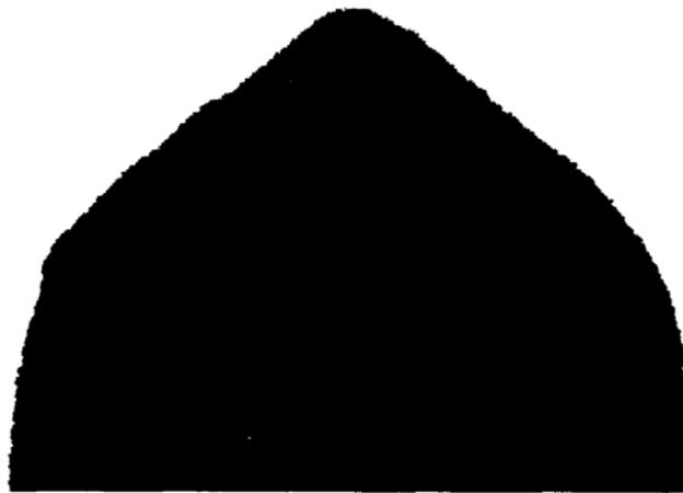
**Figure 3: Conical shape of the sample after the test with a pressure of 15 atm.**
