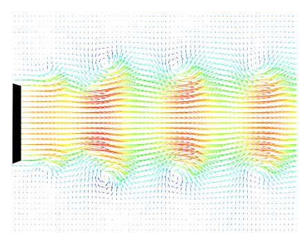
Phase averaged velocity field of excited jet (PIV measurements)
