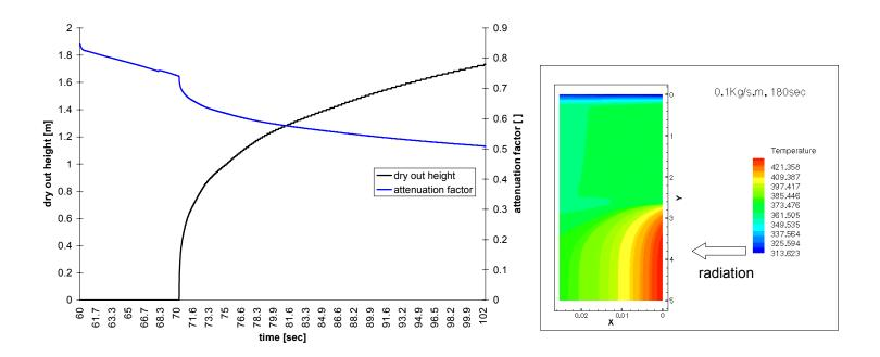
Inadequate protection with falling film (0.1kg/sm for incident radiation due to fire at 1200K)
