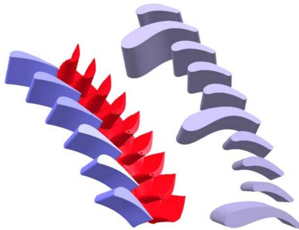
*Figure 1: First turbine stage and multi-splitter vane*
