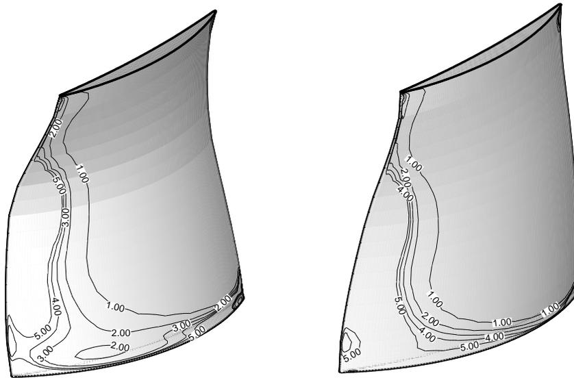
Figure 1: Loss iso-lines ( $\omega \cdot 10^5$ ) on the suction side of baseline design (right) and optimized blade (left).
