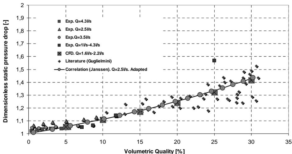
Figure 2: Evolution of the dimensionless static pressure versus the volumetric quality of air. Convergence restriction.
