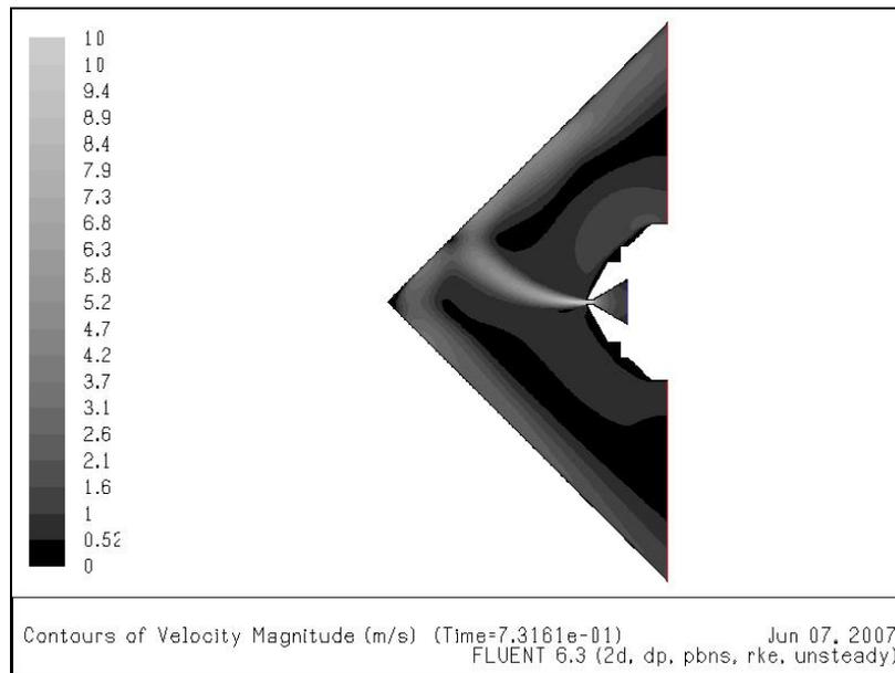
Figure 1: CFD simulation of Flapping jet
