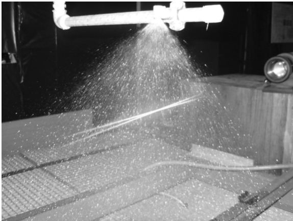
Figure 1: PDA experiments with water for the full cone nozzle; P = 800 \text{ kPa} , L = 100 \cdot d_0
