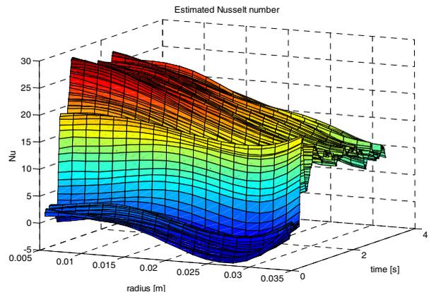
Figure 2: Inverse methodology applied to an impinging hot-air jet. Left: temperature measurement performed via IR camera along the radius of a circular plate. Right: Nusselt number evolution retrieved through inverse methodology on the opposite surface of the plate.
