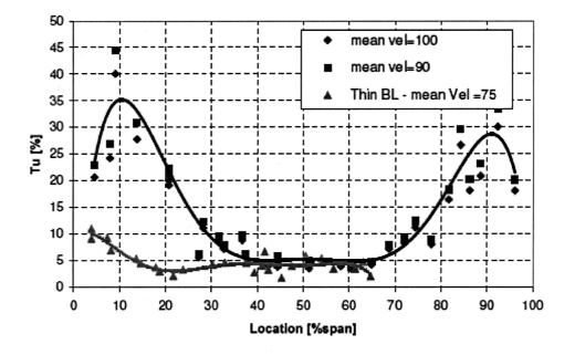
Figure 1: Turbulence intensity at the stage inlet
