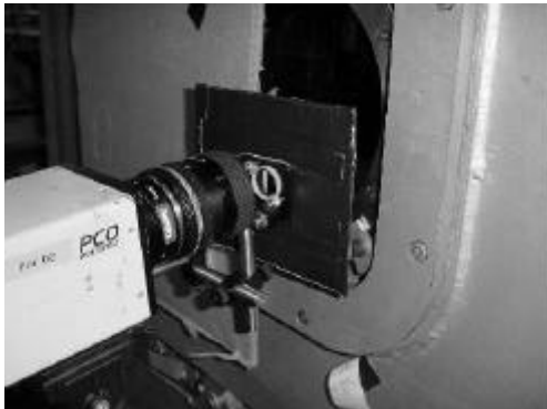
Figure 1: Optical setup at VKI H3 M=6 wind tunnel
