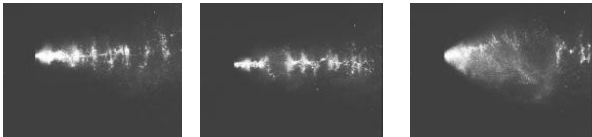
Figure 1: Instantaneous images of a flashing jet R134a
