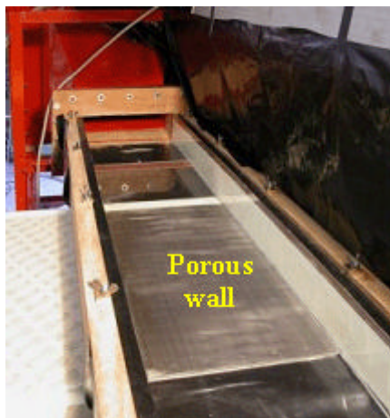
Figure 1. Test section view with the porous plate on the bottom wall
