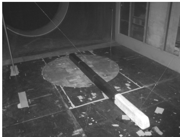
Figure 2: Picture of the model attached in L1-B wind tunnel
