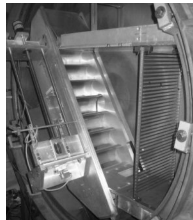
Figure 1: Left: kinetic losses against Reynolds number and classification for the separation bubbles Right: VKI S1/C cascade wind tunnel test section: T106 linear cascade and turbulence generator grid
