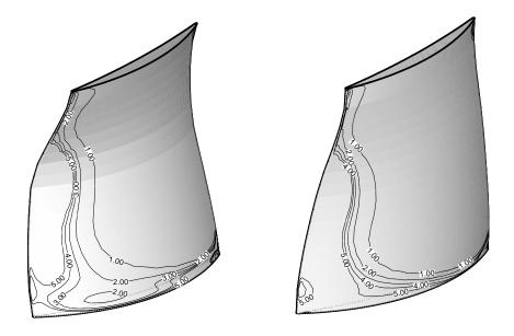
Figure 1: Loss iso-lines ( $\omega \cdot 10^5$ ) on the suction side of baseline design (right) and optimized blade (left). The trailing edge is on the left
