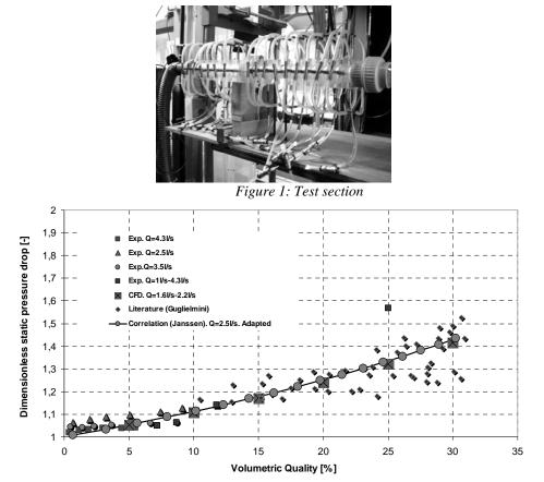
Figure 2: Evolution of the dimensionless static pressure versus the volumetric quality of air. Convergence restriction.
