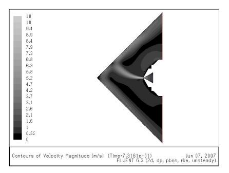
Figure 1: CFD simulation of Flapping jet
