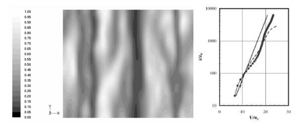
Figure 1: map of wall-shear stress (left), [Pa], traces of super-streaks; (right) normalized velocity profile, solid line LES-UDF, dashed line baseline Sullivan's model (1994).
