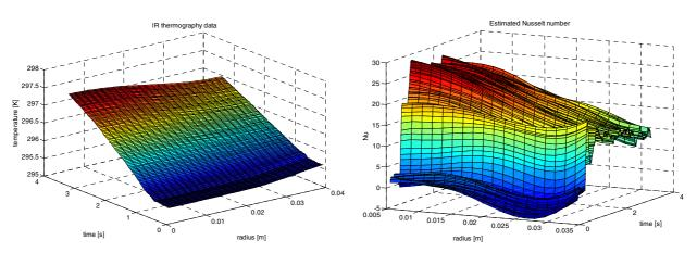
Figure 2: Inverse methodology applied to an impinging hot-air jet. Left: temperature measurement performed via IR camera along the radius of a circular plate. Right: Nusselt number evolution retrieved through inverse methodology on the opposite surface of the plate.
