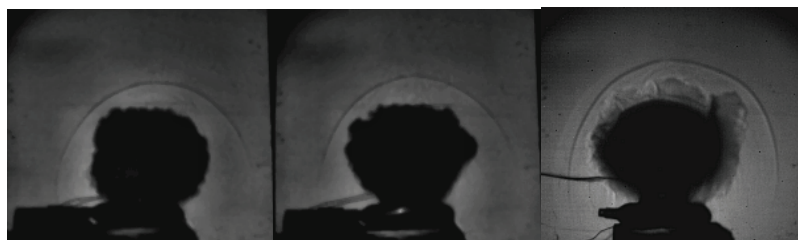
Figure 2: Shadowgraph of BLEVE rupture: 80mm weakness (left), 40mm (middle) and 10mm (right)
