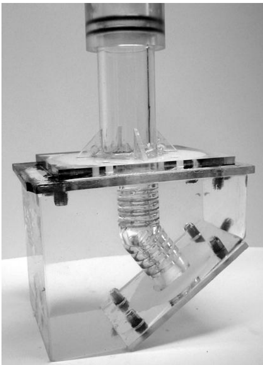
Figure 1: left: Alveolated duct model used in experiment. Right: 5\mu\text{m} particle trajectories for 22 nd lung generation, front view.
